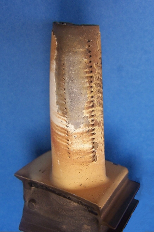
Fig. 1. Image of the leading edge of an engine-run high-pressure turbine blade showing severe foreign object damage. Note the large gray region which indicates bond coat exposed by complete removal of the TBC.
