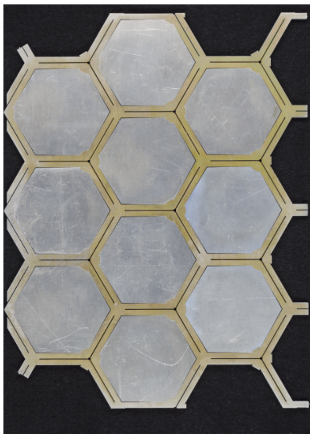
Fig. 10. Lattices of Ti alloy (struts) and Al alloy (hexagonal units) fabricated for measurement of the coefficient of thermal expansion.
