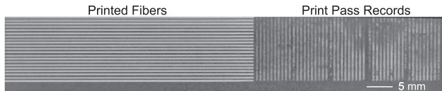
Fig. 1. As-printed ceramic microbeams. At left, beams printed by the subsequent application of 50 layers of 17 vol% alumina ink. At right, each stripe provides a record of printing success for all nozzles at each print pass.
