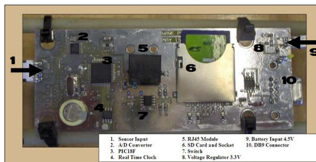
Figure 6. Fabricated Circuit Board
