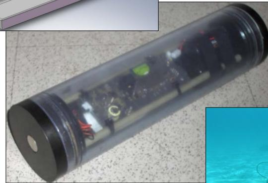
Figure 4. The Wave Height Pressure Sensor
