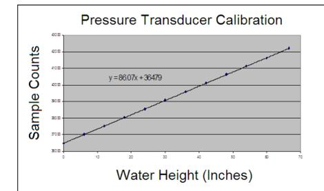
Figure 7. Linear Calibration Curve
